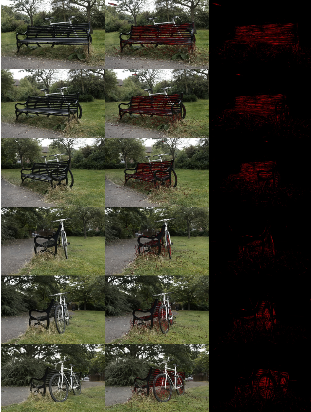
Figure 11: Rendering results of Mip-NeRF360 dataset of our method. We visualize Gaussians with effective rank smaller than 1.02 in red. Effective rank regularization is adaptive to the scene, reducing the number of needle-like Gaussians, while effectively representing the required regions.
